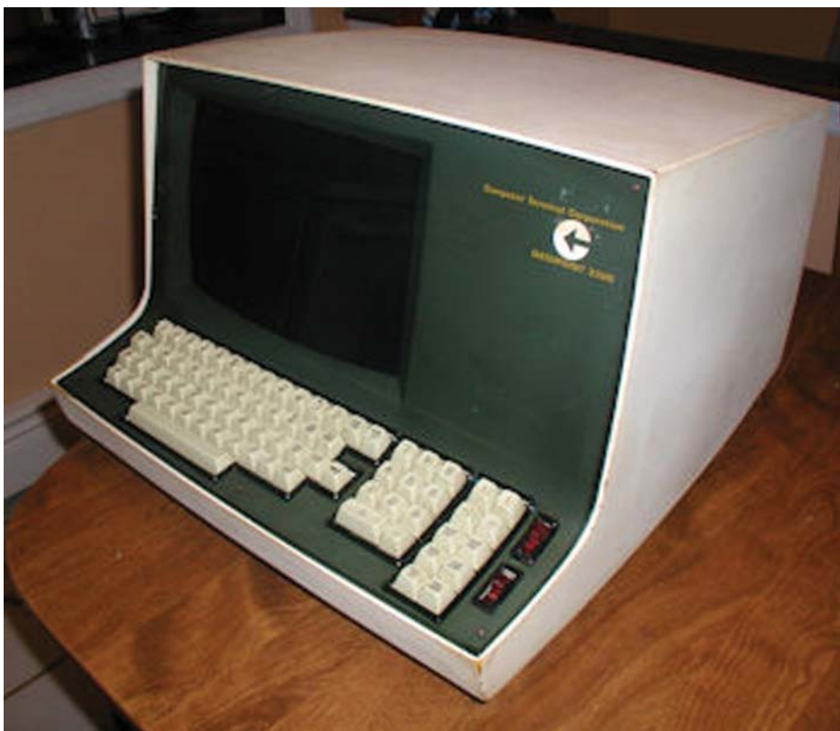
Figure A.4 Datapoint CRT terminal
